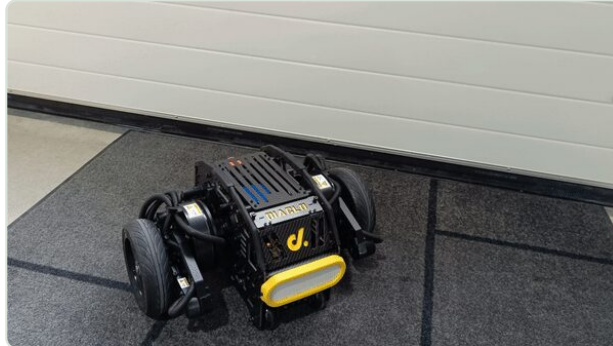
Diablo demonstrating its wheel-legged balancing and posture-change capabilities.
