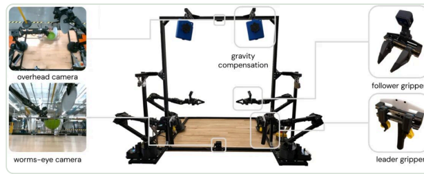
ALOHA 2 components including cameras, grippers and gravity compensation system
